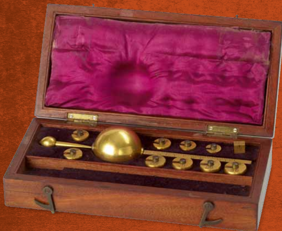
De hydrometer van Sikes.
